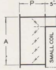
FACE & INTERNAL BY-PASS DAMPERS — FOR MOUNTING AT UPSTREAM SIDE OF COIL
